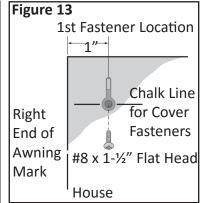
**29.** On the mark, snap a chalk level line along the entire length of the Awning. On the chalk line, mark the location of the right end of the Awning. Along the chalk line you just made, measure 1" further to the right of the Awning end point and make a mark. This is the location of the first fastener on the right for the Protective Cover. See **Figure 13**.
