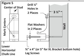
**6.** Remove the Bracket and drill the top hole through the siding block or shim (if appropriate) and about 3 ½" into the stud or joist using a ¼" drill bit. This will prevent the framing from splitting while installing the Lag Screws.
