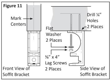
**25.** Using a %6" socket, install the Bracket with the %" x 4" Long Lag Screws. Use the Flat Washer provided under the head of the Screw. Make sure not to overtighten the Lag Screws; doing so may split the wood framing or weaken the Screw. See **Figure 11**.
