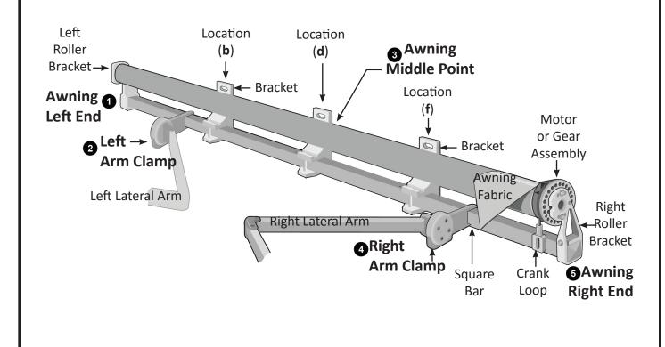
Figure 1c **Bracket Locations for 14' - 16' Wide Awnings** Location (a) Left Location - Awning Roller (b) Middle Point Bracket → - Bracket Location Awning 1 (f) **Left End** Location Motor (g) 2 Left or Gear Assembly **Arm Clamp** Awning Fabriç Left Lateral Arm Right Right Lateral Arm - Roller Bracket **4** Right Arm Clamp
