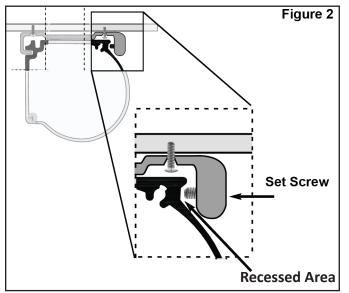
**6.** Using the <sup>1</sup>/<sub>8</sub>" Allen Wrench, tighten the Set Screw in each of the Mounting Brackets until the EasyShade Assembly is secure. See **Figure 2a**.
