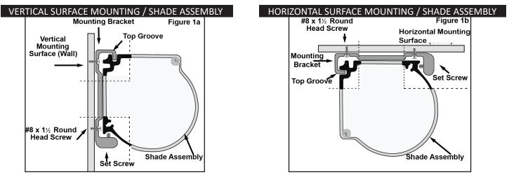
**1.** Determine the desired location for the Mounting Brackets, making sure that they are plumb and level. Using a pencil, mark the 2 Bracket hole locations on the Mounting Surface. Using a  $\frac{1}{2}$ " bit, drill holes approximately 1- $\frac{1}{2}$ " deep at both hole locations. Repeat for the Mounting Bracket on the other side, and the center Mounting Bracket location on 10' to 12' models.
