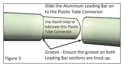
**Step 3**. The Aluminum Leading Bar for EasyShade models 9 to 12 FT long will require assembly of two sections of Leading Bars. **Note:** When connecting these two sections, ALIGN THE GROOVES in the Leading Bars. See Figure 3.
