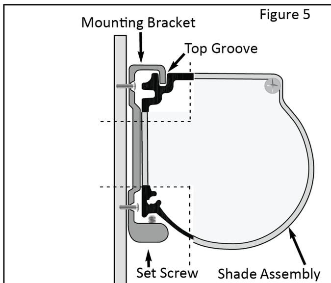
10. Tighten the set screw in each Mounting Bracket until the Shade Assembly is secure.
