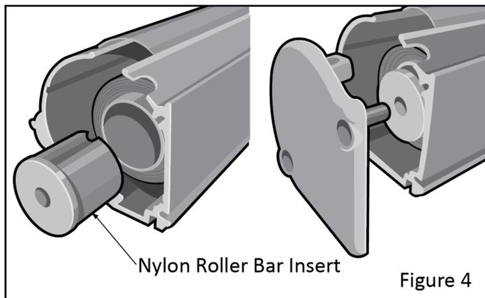
9. With your helper, lift the Shade Assembly up to the installed Mounting Brackets and insert the Top Groove of the Shade Assembly onto the protruding tab on the Mounting Brackets. While maintaining upward pressure to keep the Top Groove of the Shade Assembly on the tab of the Mounting Brackets, press the Shade Assembly toward the Mounting Bracket and be sure that the Set Screw is aligned in the recessed portion of the Shade Assembly. See Figure 5.
