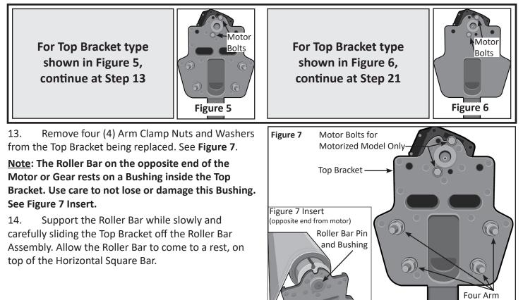
15. Remove the Top Bracket from the Arm Clamp Bracket Bolts, by slowly and carefully sliding it away from the four bolts of the two Arm Clamp Brackets. Support each Arm Clamp while they are removed from the Top Bracket, one side at a time.
