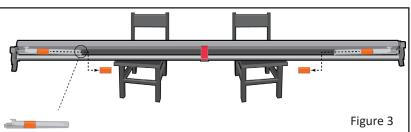
8. Remove the two nuts and bolts that attach the Square Bar Uprights to the Corner Braces, at both ends of the OASIS. <u>Note</u>: A helper should stabilize each Square Bar Upright AND the Roller Bar Assembly as they are being separated and removed. See Figure 4.
