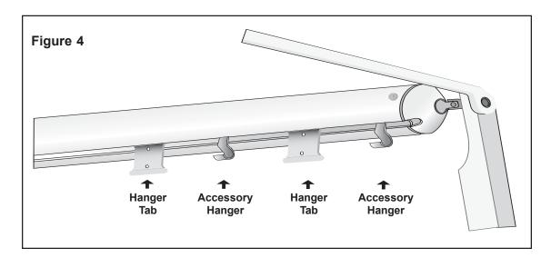
**STEP 7b.** Attach the hooks on the top of each light assembly into the bottom hole of each hanger tab.
