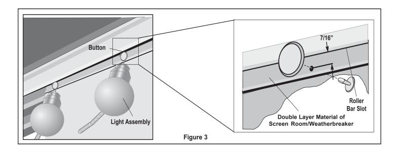
STEP 7a. Place the hook on the top of each Patio Light over the installed button. Proceed to STEP 10.
