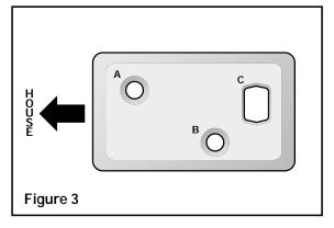
**Step 6.** Drill a clearance hole (one per plate) at point C, 3/8" deep using a 5/8" drill bit. Make sure to clean out the holes.
