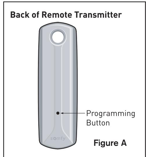
10. When the motor stops, press and hold the programming button on the back of the Remote Transmitter (see fig. A) for 5 seconds until the motor 'jogs', then release. (A 'jog' is a short back and forth movement of the motor).
